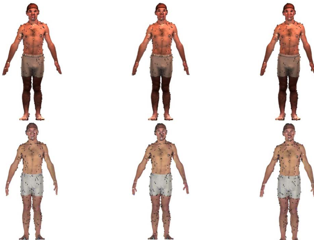
Fig.3. Automatically selected intrinsic landmarks of a subject, where the black dots mark selected landmarks, found in all six scans. The white dots are clothing industry standard landmarks, physically marked on the subjects prior to scanning.
