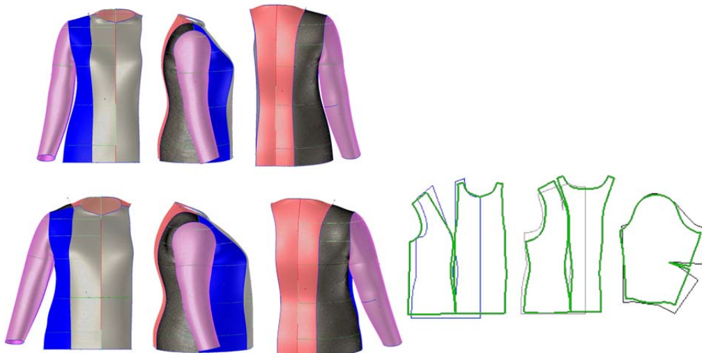
Fig. 10: Left: Blouse construction in 3D, right: 2D pattern parts
